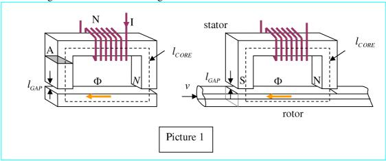
The magnetic reluctance of the iron core and the magnetic reluctance in air gap in picture 1 are;
