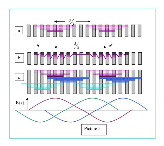
The flux density B(x) became time dependent B(x,t) if the DC current is replaced with a time dependent current i(t)
