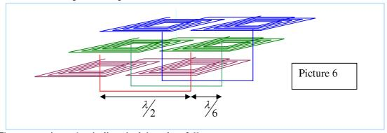
The current in each winding is delayed as follows
