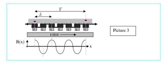
to make flux destiny B(x) sinusoidal the stator is wounded in a sophisticated manner, as shown in picture 4. Windings wires are pushed into slots as seen in picture 5. Two winding option  $\bf{a}$  and  $\bf{b}$  are equivalent but in machine industry,  $\bf{a}$  is preferable. picture 5-c describe windings in a 3 phase machine, and will be discussed later.
