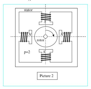
In rotating machines we have a moving part; the rotor and a static part; the stator. The rotor and stator have the same principles of operation.
