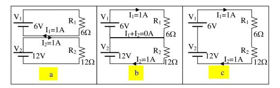
In figure-a, two separated DC sources are connected to two separated resistors, the current in each resistors can be checked to be 1A and the number of wires required to connect the two resistors to both DC voltage source is four.
