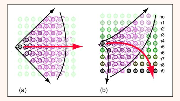
FIG. 10 (a) A light wave radiates in vacuum of index of refraction n<sub>o</sub>=1 (b) In an inhomogeneous potential field of variable index of refraction the wave is distorted accordingly by refraction. Particles (not shown) having the same momentum and traveling in the same media would be similarly 'refracted' (large arrows).
