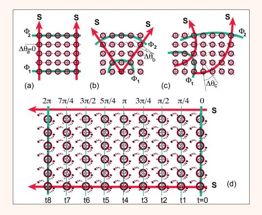
FIG. 7. Fields in (BU) can be in equilibrium (a), (b), (c), or time varying radiation fields (d). In all cases equipotential surfaces ( $\Phi$ ) are where node-to-node orientation  $\Delta \theta$  is constant. Streamlines (S) are normal to ( $\Phi$ ). (d) The nodes in a radiation field transfer angular momentum along (S) so that nodes on successive ( $\Phi$ ) have different phase angles  $\theta$  at various times t0,t1,t2,
