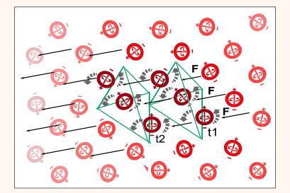
FIG. 19 Motion of a particle across a lattice of nodes: the nodes themselves do not move, only their pattern of spin. At time t1 the particle at right experiences new momentum impinging on it as a force (F) The particle's spin pattern is translated to its new position at time t2. The surrounding gravitational field nodes' pattern (left) experiences a similar transfer in position
