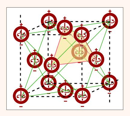
FIG. 4 Self-assembly of magnetic dipole nodes oriented in the same direction as a Face Centered Cubic (FCC) Kepler packing. Each unit of the packing forms a cube with a node at each corner, with another node where the cube's diagonals cross. The smallest regular volume made up of four nodes would be a tetrahedron (shaded).
