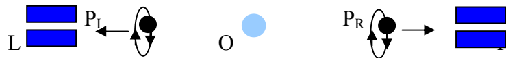
The experimental set up involves emitting of two spin \frac{1}{2} particles P_L and P_R having opposite spin states from a system at O . Two detectors L and R kept at a large distance from each other measures the spin state of the particles at the same instant.
