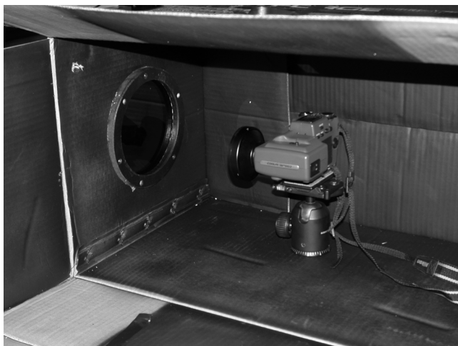
Figure 6: The experimental setup showing camera in a box and lens on the left face of the box. During operation, the box is closed, and the room lights usually turned off.
